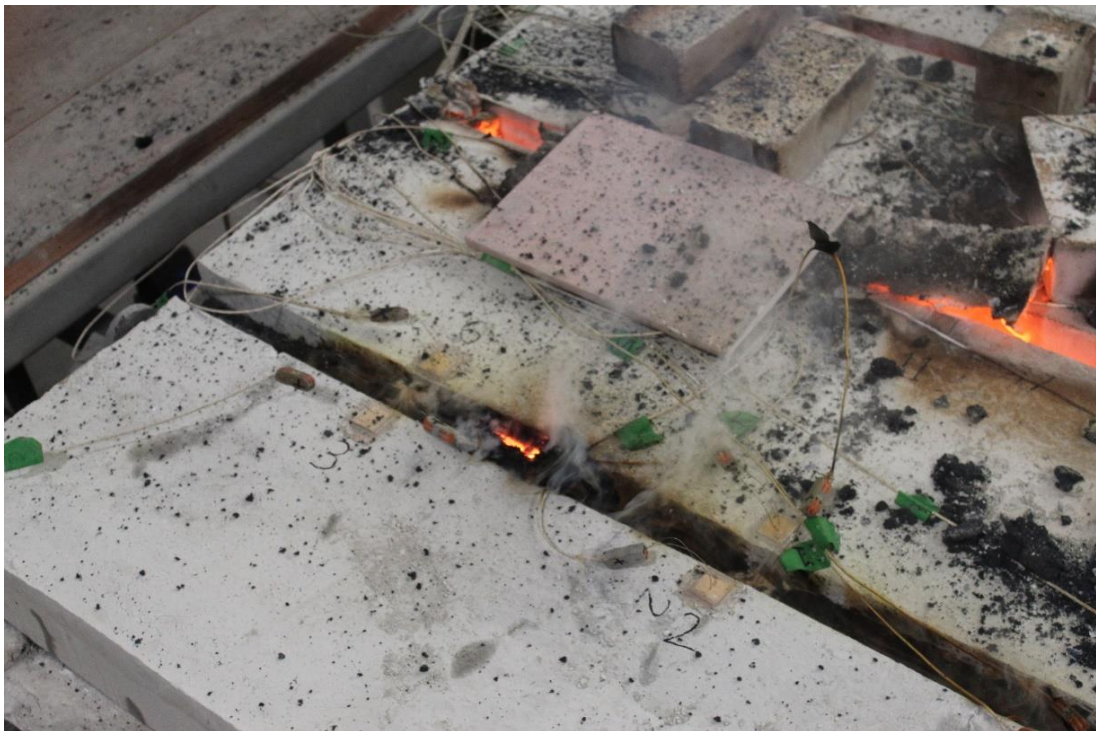
Specimen A - Small visible red spot in seal – 76 Minutes
